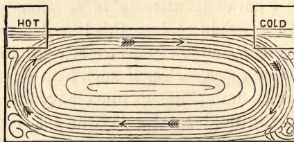
Fig. 170.—Ex.—Dr. Carpenter's, showing Circulation of Water by Thermal Forces.
